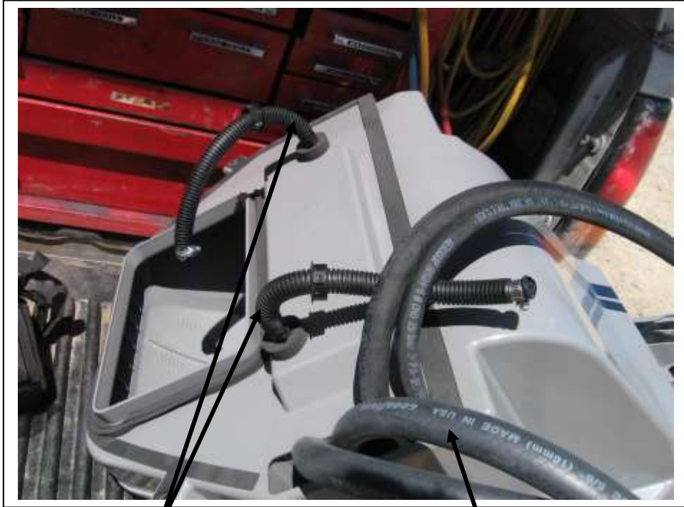
Drain tubes installed
