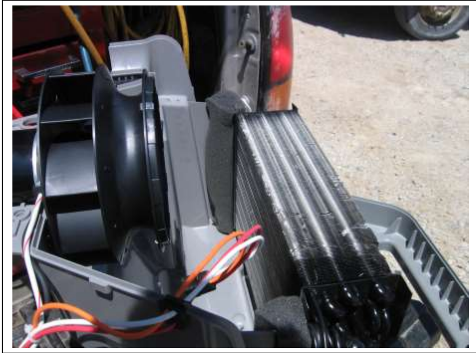
Heat/cool coil in place with hoses attached. Seal coil in box with foam or tar tape.
